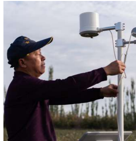
XAG Agriculture IoT device powered by solar panels
