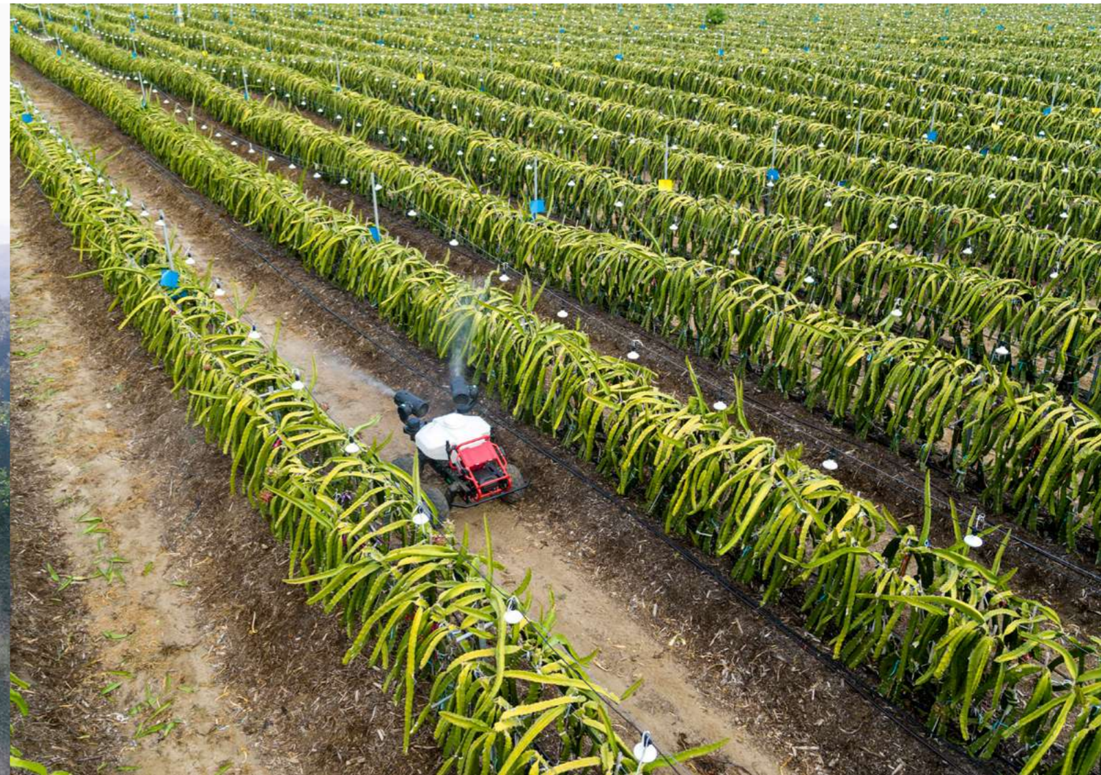
Plant protection in dragon fruit orchard by XAG R150 Unmanned Ground Vehicle
