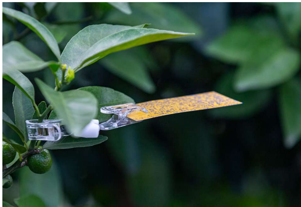
Use water-sensitive paper to measure the quality and pesticide utilization rate of drone spraying
